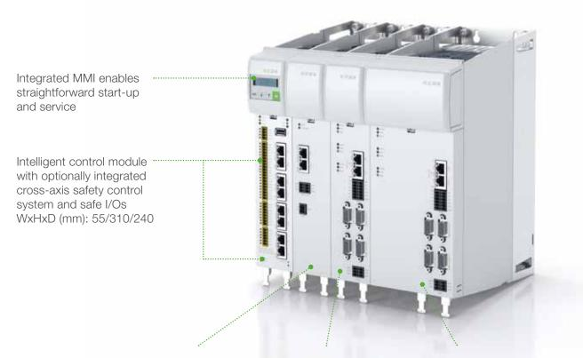
Energy-efficient power supply module, optionally regenerative WxHxD (mm): 55/310/240 Drive module for continuous motor currents from 1.5 A to max. 12 A WxHxD (mm): 55/310/240 Drive module for continuous motor currents from 12 A to max. 24 A WxHxD (mm): 110/310/240
